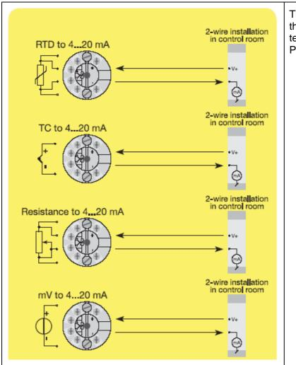
The temperature sensing devices that can be connected to the temperature transmitter PR5337 / PR6337 with 4..20 mA output are:
